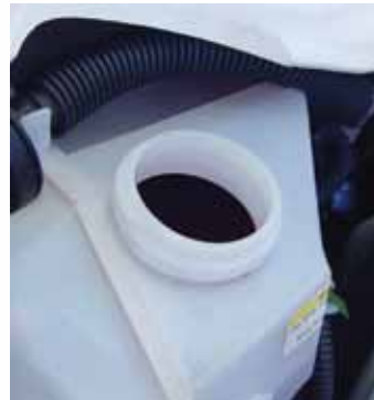
Oil Sleeve NOT installed
