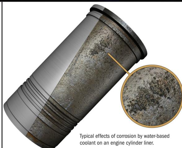
Typical effects of corrosion by water-based coolant on an engine cylinder liner.
