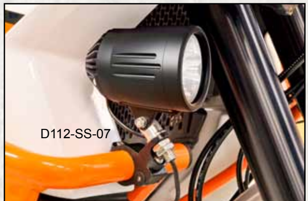
70mm LED mounted on KTM 990 Adventure pg. 26
